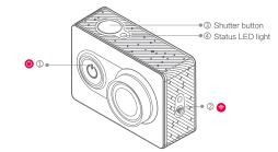
1) Turn on the camera: Click on the Power/Mode button. The LED light will blink few times. Turn off the camera: Press the Power/Mode button for 3 seconds. The LED light will blink 7 times
